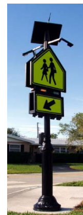
Rectangular Rapid Flash LED Beacon (RRFB)
